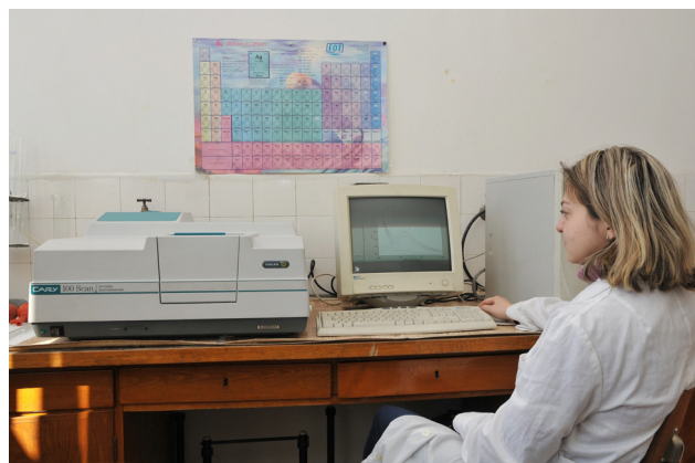
photometer, model “Cary -100” of the company “VARIAN” having spectral bandwidth of (190-900 nm), dual channel FTIR
